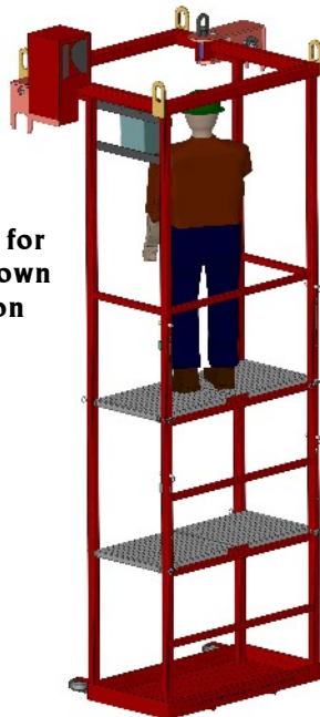
Powered drive for traversing and fold down steps for elevation
